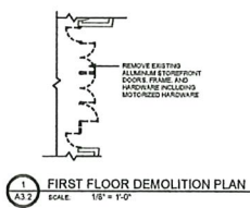
1 FIRST FLOOR DEMOLITION PLAN SCALE: 1/8" = 1'-0"
